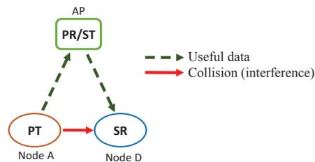
Fig. 2. Inter user interference in FD-WLAN
