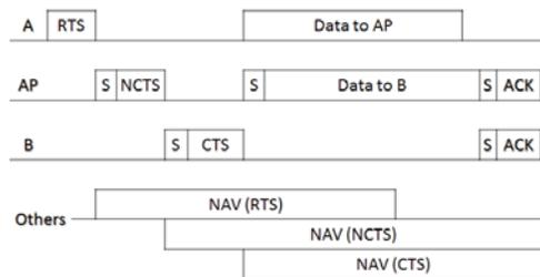
Fig. 3. HDN Starts Transmission: Case-1
