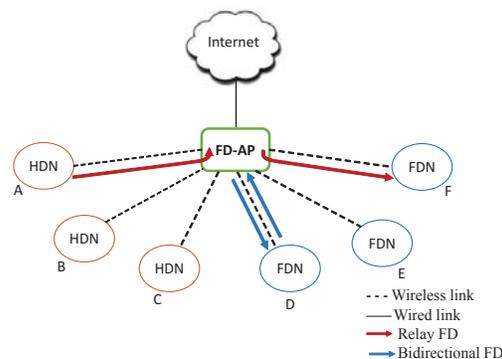
Fig. 1. Structure of a Het-WLAN
