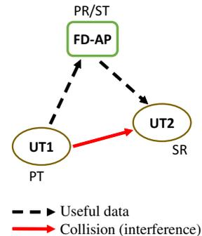
Fig. 2. Inter user interference in IBFD wireless LAN.
