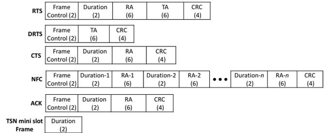
Fig. 5. Format of control frames (in octet).
