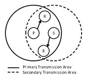
Fig. 2. Collision between a primary transmission and a secondary transmission
