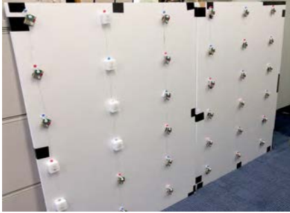
Fig. 9. Prototyped IR-sensor Array for Motion Detection
