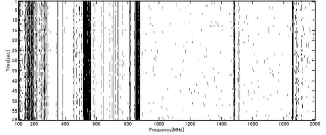
Fig. 8. Real spectrum utilization data.
