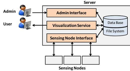
Fig. 4. Server software components
