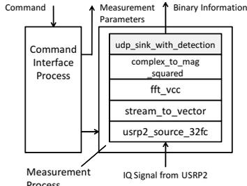
Fig. 18. Process and GNU Radio signal processing block diagram
