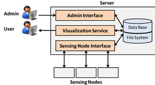
Fig. 4. Server software components
