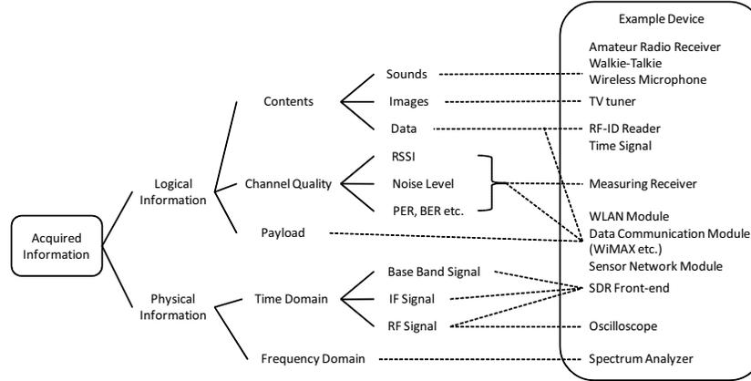
Fig. 9. Classification of information generated from various wireless devices and measurement equipment.
