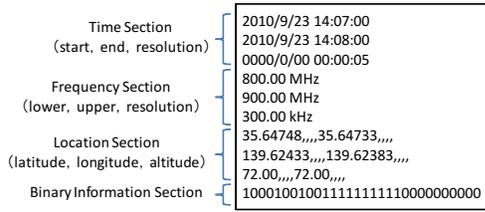
Fig. 5. TSF (Tiny Spectrum Format)
