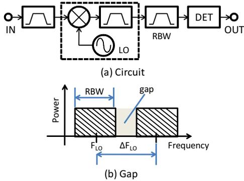
Fig. 15. Measurement using a spectrum analyzer
