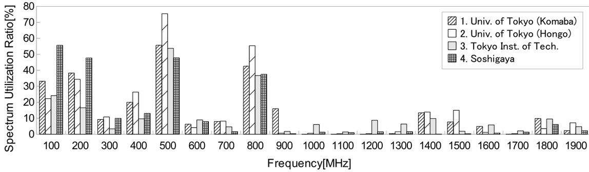
Fig. 25. Spectrum utilization ratio at 4 locations
