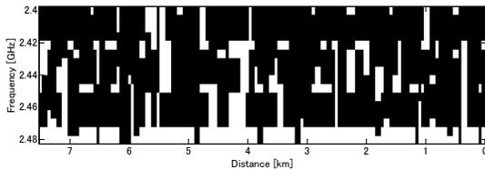
Fig. 27. Spectrum utilization along a route
